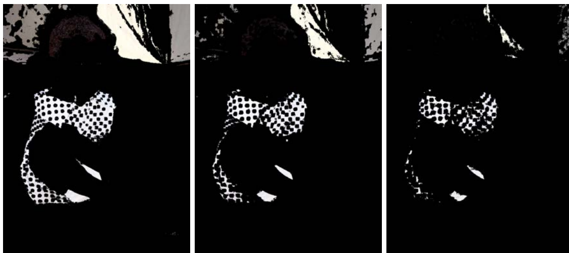
Figure 3.50: Predicted non-skin with 66%, 95%, 99.5% confidence. Non-skin is harder to detect due to its variety.
